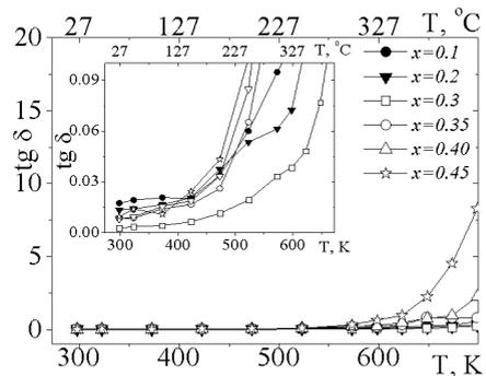
Fig. 5. The tgδ vs temperature curves of Sr<sub>1-1.5x</sub>Bi<sub>x</sub>MoO<sub>4</sub> compositions at 1 kHz
