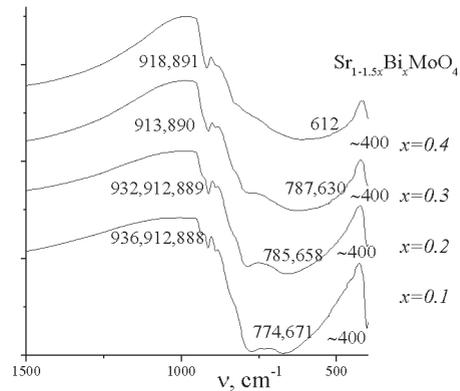
Fig. 3. IR FT spectra of the  $\text{Sr}_{1-1.5x}\text{Bi}_x\text{MoO}_4$  compositions
