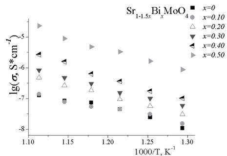
Fig. 4. Arrhenius plots for selected Sr<sub>1-1.5x</sub>Bi<sub>x</sub>MoO<sub>4</sub> compositions
