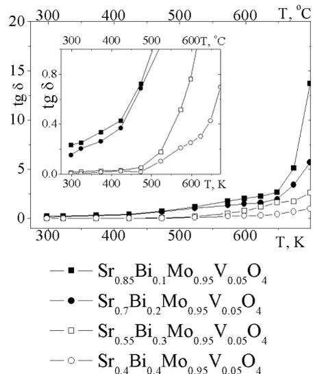
Fig. 6. The tgδ vs temperature curves of several Sr<sub>1-1.5x</sub>Bi<sub>x</sub>Mo<sub>1-y</sub>V<sub>y</sub>O<sub>4-d</sub> compositions at 1 kHz
