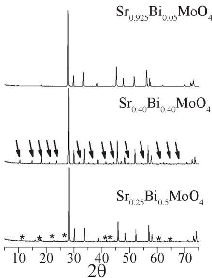
Fig. 1. X-ray diffraction profiles for selected  $\text{Sr}_{1-1.5x}\text{Bi}_x\text{MoO}_4$  compositions. Arrows and asterisks indicate superlattice and  $\text{Bi}_2\text{Mo}_3\text{O}_{12}$  reflections, respectively
