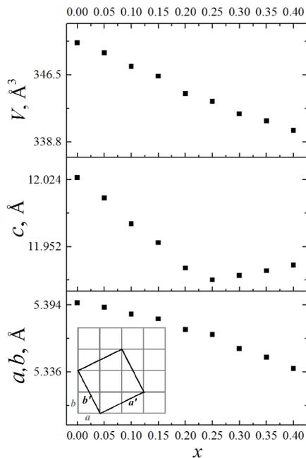
Fig. 2. Compositional variation of unit cell parameters in  $\text{Sr}_{1-1.5x}\text{Bi}_x\text{MoO}_4$ ; super ( $a', b'$ ) and sub ( $a, b$ ) — cells in  $\text{Sr}_{1-1.5x}\text{Bi}_x\text{MoO}_4$  series (inset)
