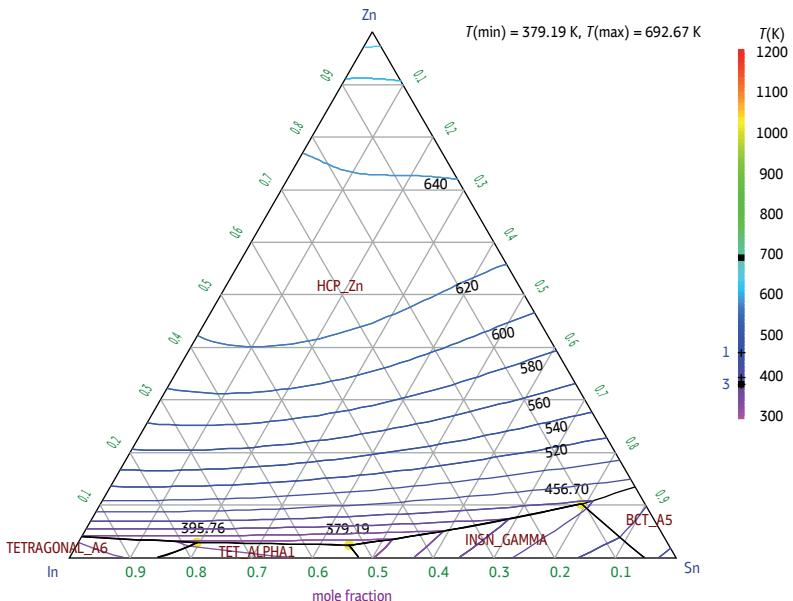
Fig. 4. Calculated liquidus surface in the In-Sn-Zn system
