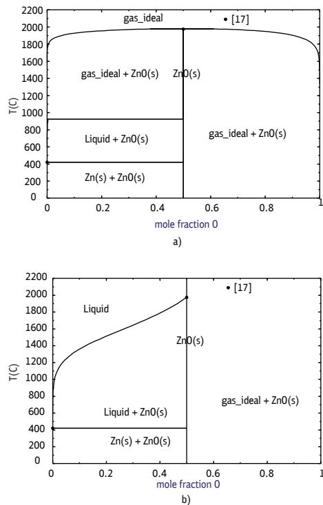
Fig. 8. Calculated Zn-O phase diagram:
