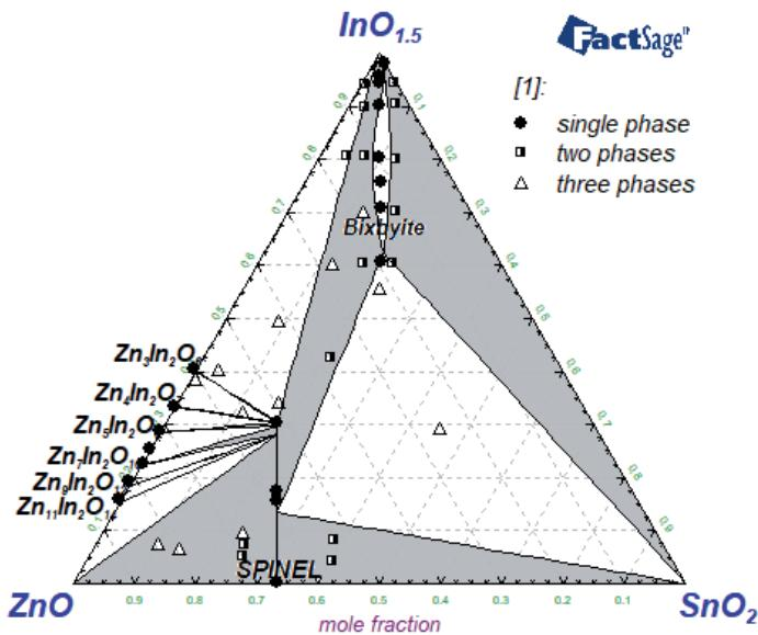
Fig. 18. Subsolidus phase relationships in  $\text{In}_2\text{O}_3$ - $\text{SnO}_2$ - $\text{ZnO}$  system in air at 1275 °C and 1 atm compared with experimental data [1]. Grey areas are the two-phase regions
