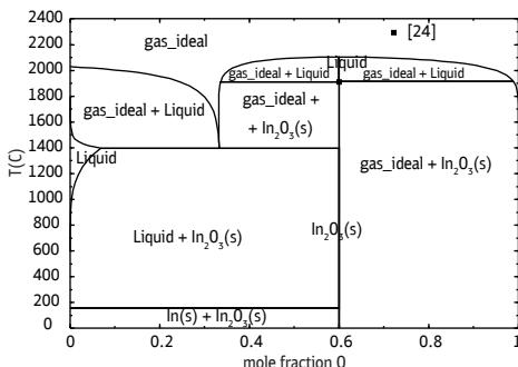
Fig. 5. Calculated In-O phase diagram
