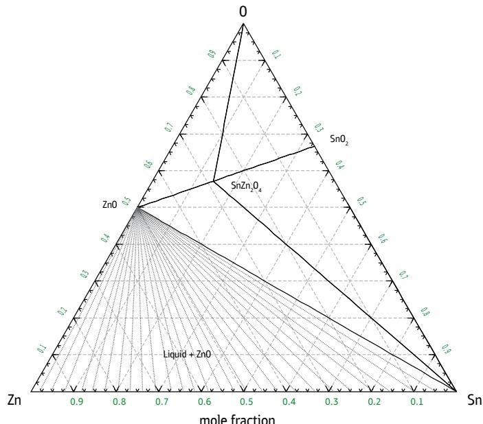
Fig. 12. The calculated Sn-Zn-O isothermal section at 500 °C
