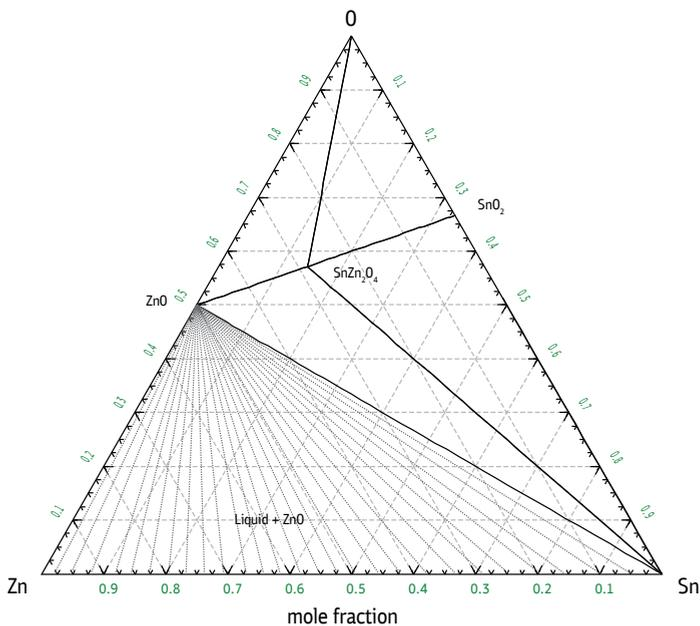
Fig. 12. The calculated Sn-Zn-O isothermal section at 500 °C
