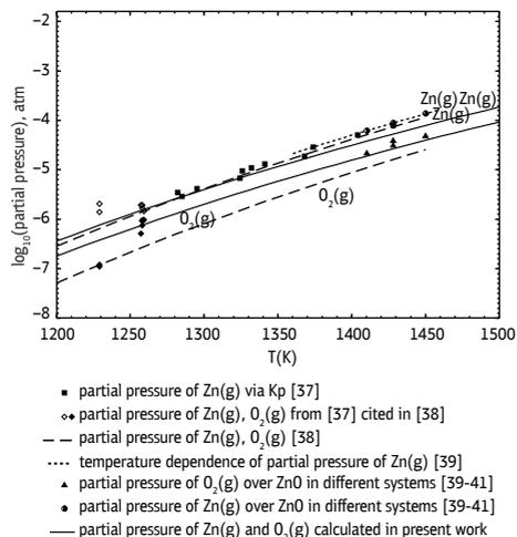
Fig. 9. Partial pressure of Zn and O<sub>2</sub> over ZnO: comparison of literature data (points, dashed, dotted lines) with calculations solid (lines)
