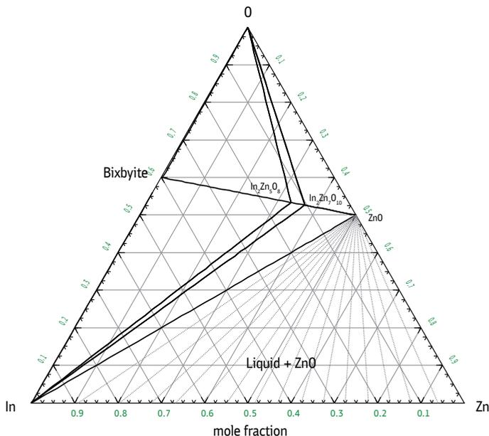
Fig. 11. The calculated In-Zn-O isothermal section at 500 °C
