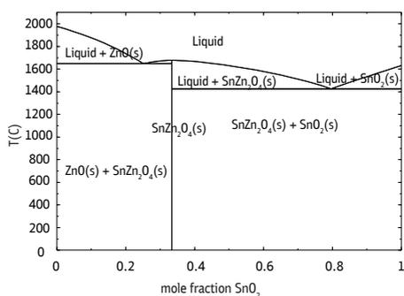
Fig. 16. Calculated  $\text{SnO}_2$ - $\text{ZnO}$  phase diagram in air
