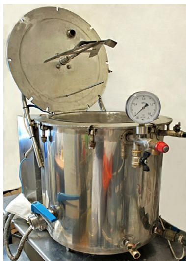
Fig. 1. The BR-30 bioreactor to produce liquid live probiotics
