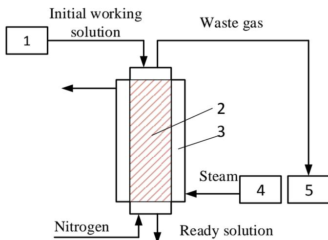
**Fig. 1** Scheme of an experimental laboratory installation: 1 - a tank for preparing the working solution; 2 - a reactor with loaded copper chips; 3 - a jacket for heating the reactor; 4 - a steam generator; 5 - an absorption tank
