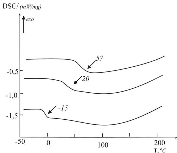
**Fig.3** DSC curves of ChT films obtained from initial solutions in the presence of glycerol with a concentration of 0, 0.05 and 0.15 mol/l (from top to bottom)
