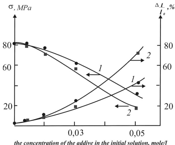
**Fig. 5** Dependence of the breaking stress and breaking elongation of films based on the ChT- glycerol (1) and ChT-propylene glycol (2) systems on the concentration of the modifying additive in the initial solution
