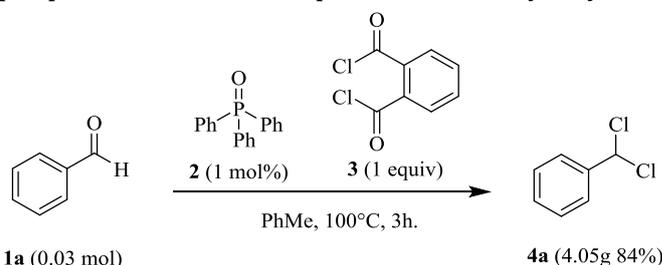
**Scheme 4** Gram-scale application of deoxydichlorination of benzaldehyde catalyzed by triphenylphosphine oxide
