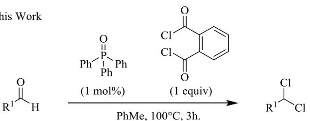
**Scheme 1** Catalytic deoxydichlorination of aldehydes to 1,1-dichlorides
