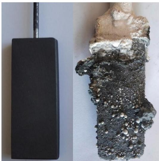
**Figure 6** Uncoated graphite cathode before and after aluminum electrolysis in vertical cell.
