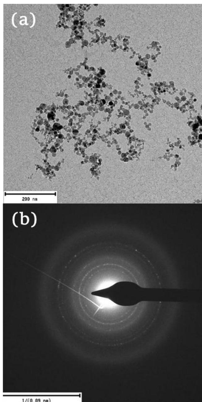
**Figure 1** Transmission electron microscopy: general view of  $\gamma\text{-Fe}_2\text{O}_3$  LTE nanoparticles (a), TEM microdiffraction confirming spinel structure (b).
