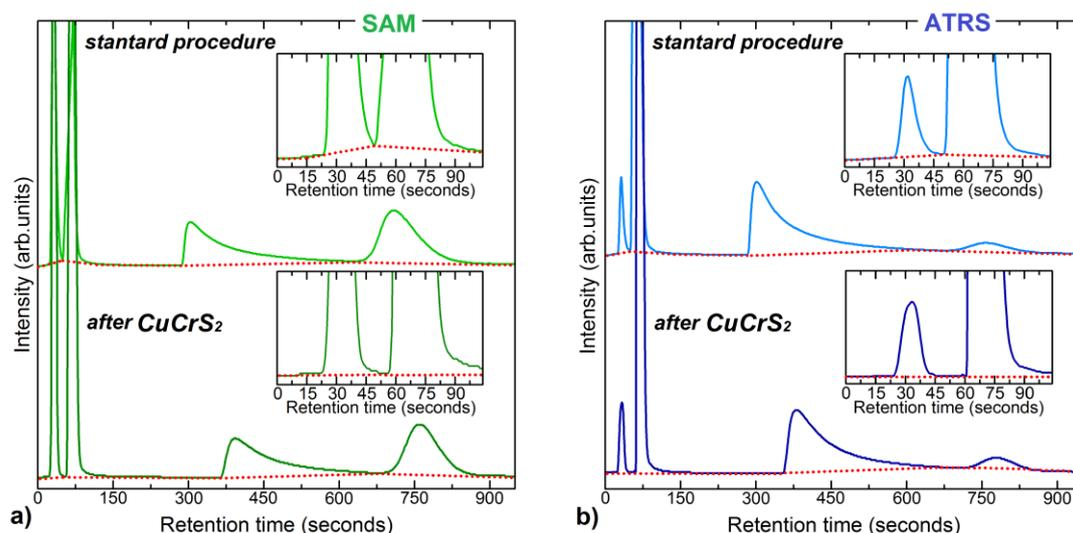
**Figure 2** Chromatograms: SAM (green solid line) after standard procedure of GCC regeneration and after  $\text{CuCrS}_2$  analysis (a); ATRS (blue solid line) after standard procedure of GCC regeneration and after  $\text{CuCrS}_2$  analysis (b). Baselines are shown as dotted red line. In the top right-hand corners, there are the insets showing the nitrogen and carbon dioxide peaks separation at a larger scale.
