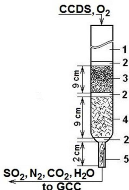
**Figure 1** Scheme of reactor for sample decomposition: pyrolysis zone (1); separation zone (quartz wool) (2); oxidation zone (3); reduction zone (4); halogen capture zone with silver wire (5).
