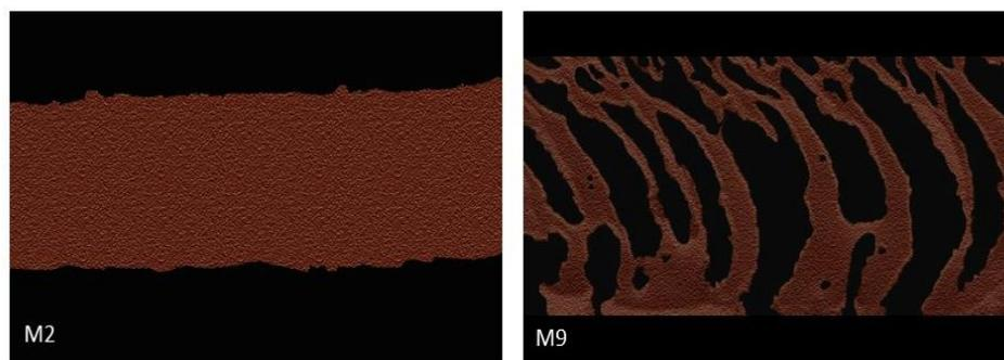
**Figure 4** The cross-sectional SEM images of prepared membranes.
