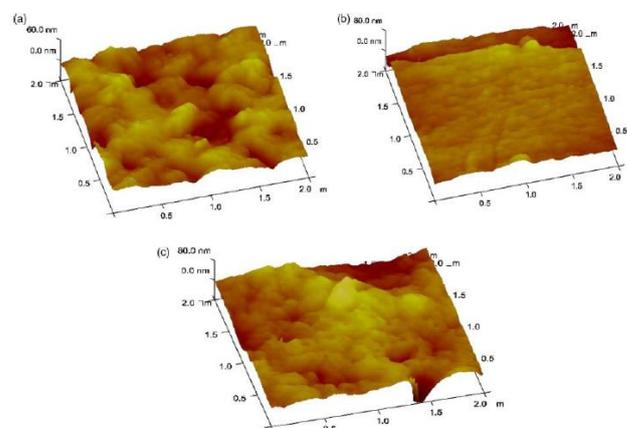
Figure 8 AFM analysis on UF membrane: (a) new UF membrane, (b) membrane contaminated with oil and (c) membrane contaminated with oil and LAS. Reproduced from ref. [35] © IWA Publishing 2007.
