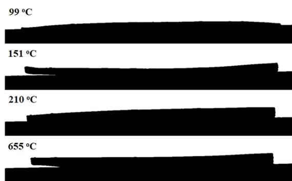
**Figure 3** Optical micrographs of LLZ film during heating (2 °C min<sup>-1</sup>).
