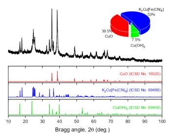
**Figure 2** XRD pattern collected from the CuHCF sample, accompanied by the reference patterns from ICSD No. 16025, No. 99499, and No. 68459.
