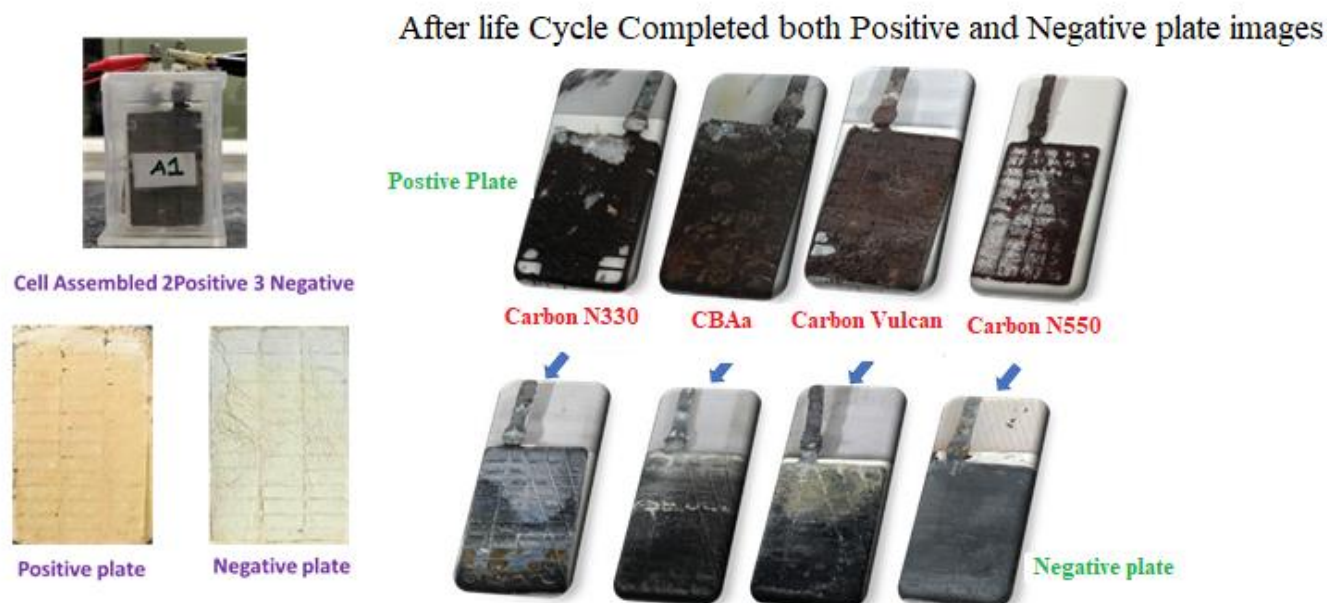
Figure 8 Plate issues and after life cycle performances following voltage drops.
