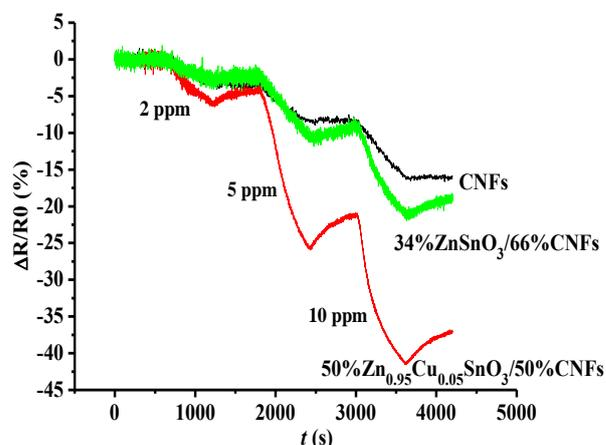
**Figure 4** Sensor response of zinc stannate-based sensor to  $\text{NO}_2$  ( $25 \pm 1\text{ }^{\circ}\text{C}$ ).
