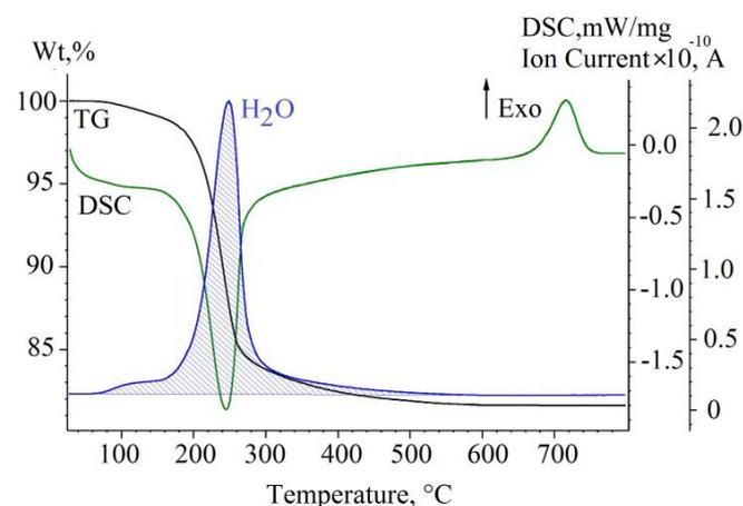
**Figure 3** Synchronous thermal analysis curves obtained during thermal decomposition of the initial sample: mass change (TG), thermal effects (DSC), and ion current of the  $m/z = 18$  amu, corresponding to water molecules released from the sample.
