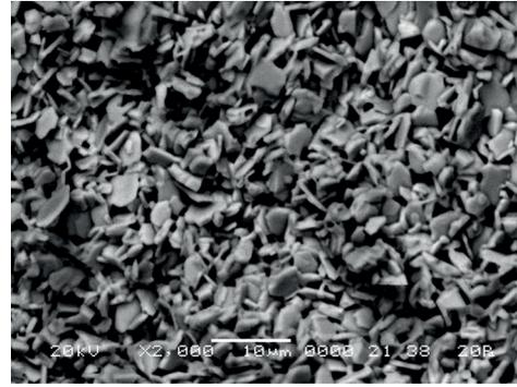
Fig. 1. Electron microscopy image of the  $\text{Ba}_{1.9}\text{Sr}_{0.1}\text{Co}_9\text{O}_{14}$  ceramics surface
