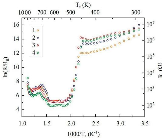
Fig. 2. The resistance dependence of  $\text{Cd}_{0.02}\text{Pb}_{0.98}\text{S}$  (1),  $\text{Cd}_{0.03}\text{Pb}_{0.97}\text{S}$  (2)  $\text{Cd}_{0.04}\text{Pb}_{0.96}\text{S}$  (3),  $\text{Cd}_{0.05}\text{Pb}_{0.95}\text{S}$  (4) solid solutions films on the heating temperature in air
