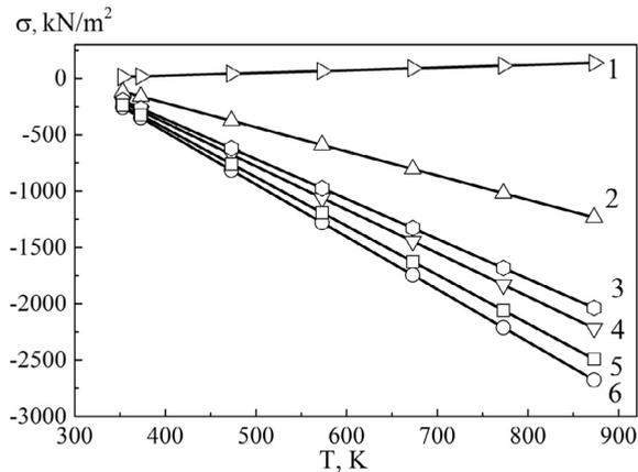
Fig. 4. Elastic mechanical stresses dependence in the systems “film — sittal substrate” on the annealing temperature in air for CdS(1), PbS (2),  $\text{Cd}_{0.03}\text{Pb}_{0.97}\text{S}$  (3),  $\text{Cd}_{0.02}\text{Pb}_{0.98}\text{S}$  (4),  $\text{Cd}_{0.05}\text{Pb}_{0.95}\text{S}$  (5),  $\text{Cd}_{0.04}\text{Pb}_{0.96}\text{S}$  (6) films
