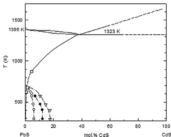
Fig. 1. Effect of the annealing temperature on the composition of  $Cd_xPb_{1-x}S$  supersaturated solid solutions in the range 403–673 K and correspondence of obtained data to the equilibrium phase diagram of the CdS — PbS system. Initial content of CdS in solid solution samples at 298 K, mol.%,: 6.0 (○), 12.2 (●), 17.6 (▽) 17.6. The duration of the annealing was 1 hour. Phase equilibrium diagram of CdS — PbS is given according to [17], dash line denotes extrapolated data [17]
