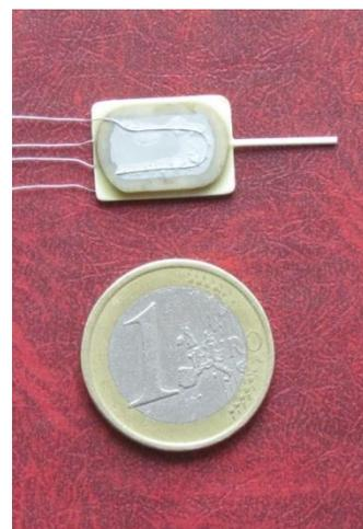
**Figure 2** General view of the sensor before the tests (the sensor appearance after 8000 h tests remained unchanged).
