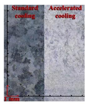
**Figure 6** Photographs of the AK6 alloy without zirconium, obtained at different cooling rates: 1 - standard;  $2 - 10^3 \text{ K/s}$ , obtained by optical microscopy.
