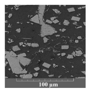
**Figure 2** Microphotograph of Al-Zr alloy containing 10 wt. % Zr.
