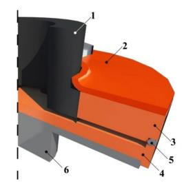
**Figure 1** Scheme of the rapid quenching installation: 1 – graphite supercharger; 2 – pressure disk; 3 – upper cooling disk; 4 – lower cooling disk; 5 – external sealing ring; 6 – electric motor flange.
