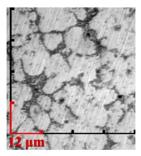
**Figure 8** Microphotograph of the AK6 alloy with a Zr content of 0.5 wt. %, obtained at a cooling rate of 10<sup>3</sup> K/s.
