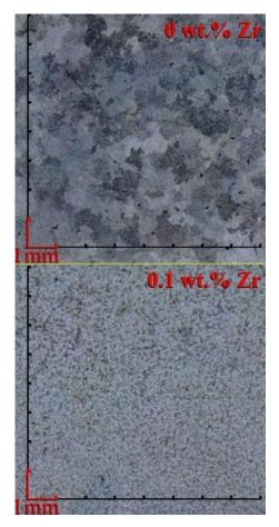
**Figure 5** Photographs of the AK6 alloy without the addition of zirconium and with a zirconium content of 0.1 wt. %, obtained by optical microscopy.
